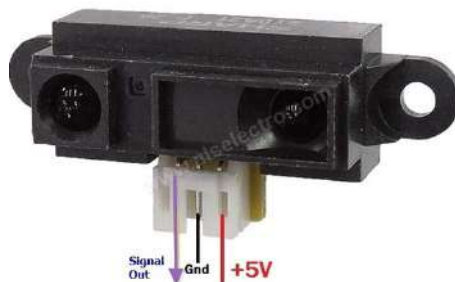
Figure 3.8: Three pins of the sensor.
