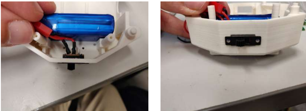
Figure 4.15: Placement of the general switch.
