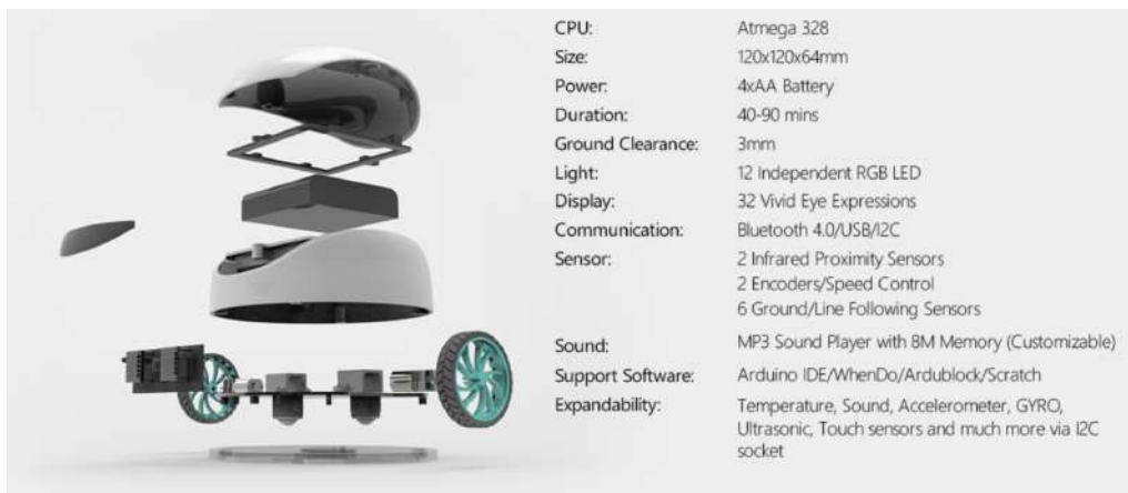
Figure 1.7: Main electronic characteristics and components of the robot.
